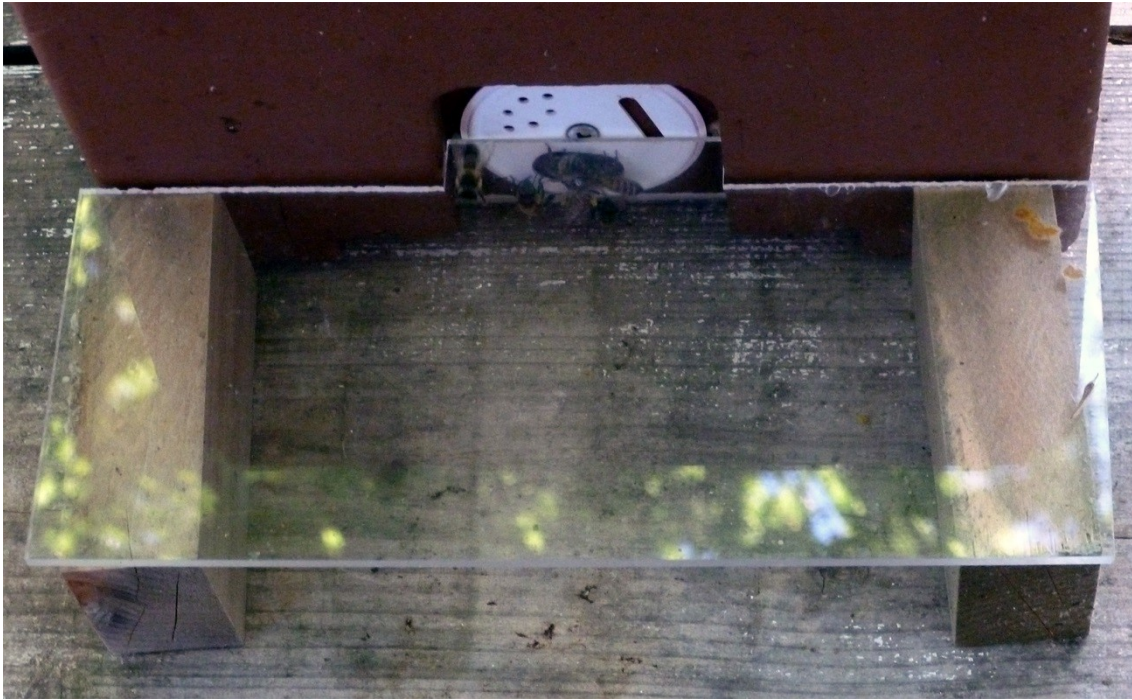
Fig. 2 Hive entrance with a lucent tunnel device for the observation of flight behavior
